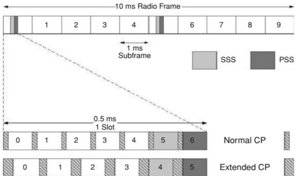
Figure 3: The PSS and SSS in the radio frame structure in the TDD frame (Sesia, Toufik, & Baker, 2011).
