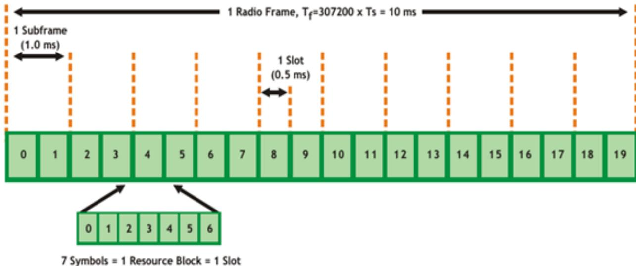
Figure 2: Time Division duplexing radio frame (Anritsu, 2009)
