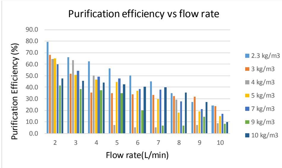
Figure 3.15: Variation of purification efficiency with stocking density at different flow rates.
