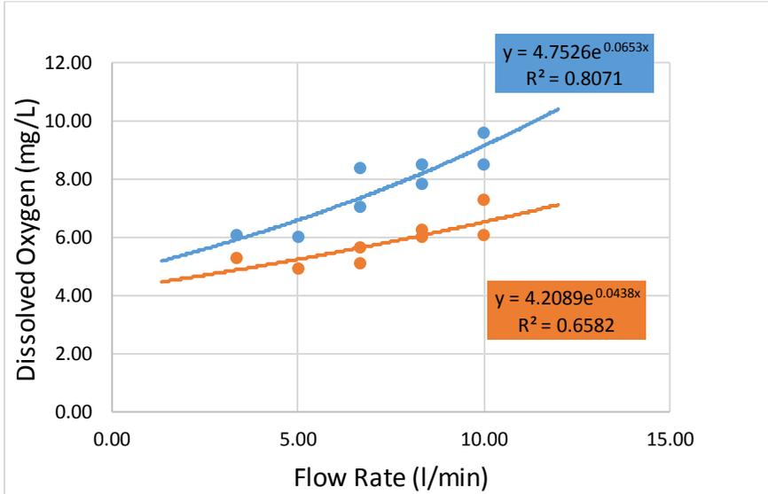
Figure 3.7: Variation of dissolved Oxygen with flow rate at 2.3kg/m<sup>3</sup> stocking density
