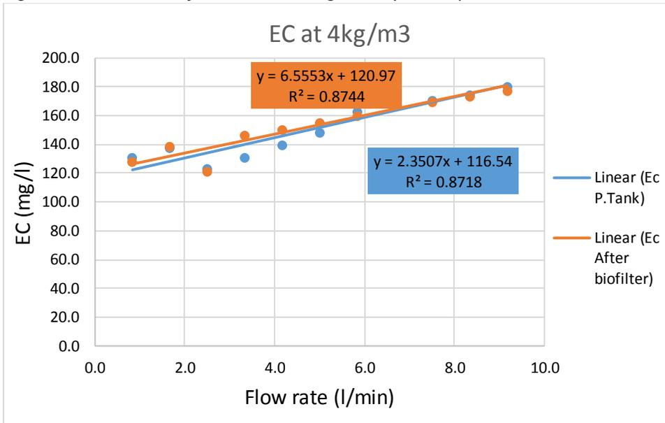
Figure 3.9: Variation of electrical conductivity with flow rate at 4kg/m3 stocking density.
