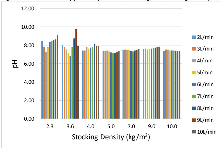
Figure 3.11: Variation of pH with stocking density in the production tank.
