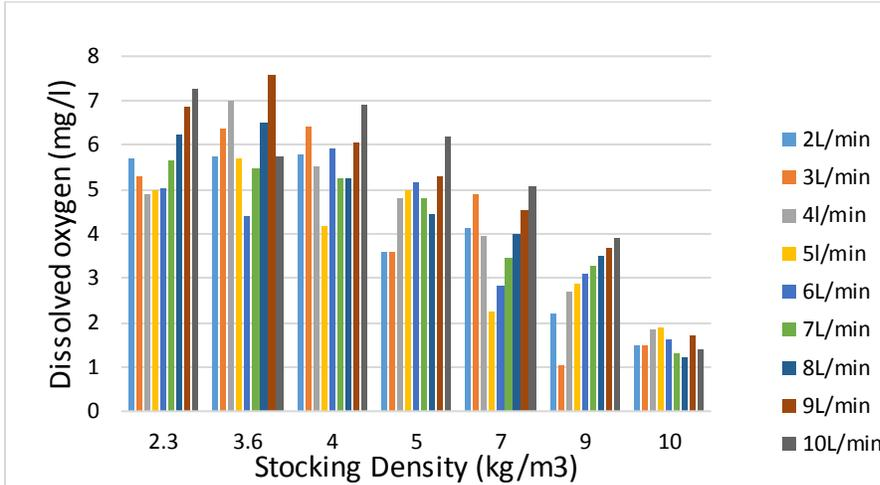
Figure 3.6: Variation of dissolved oxygen with stocking density in the biofilter.
