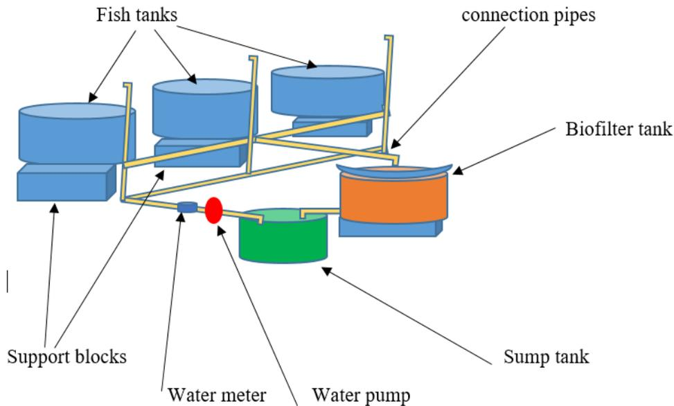
Figure 2. Error! No text of specified style in document. .2: A layout of the RAS components for a single set up.
