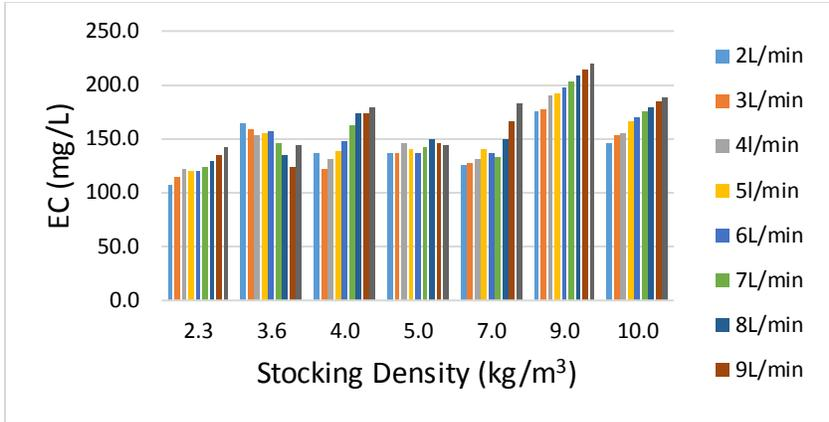
Figure 3.8: Variation of EC with stocking density in the production tank
