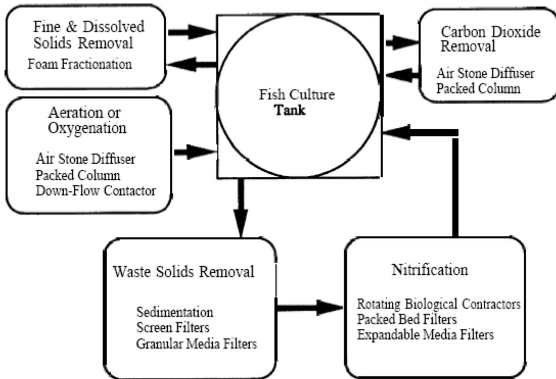
**Figure 1.** Error! No text of specified style in document. .1: A typical layout of an intensive RAS with all system components
