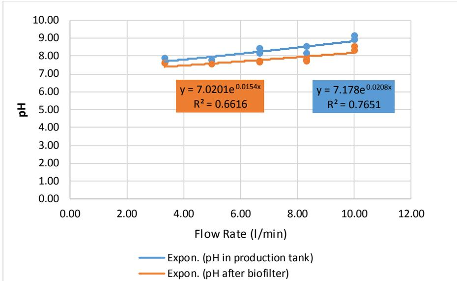
Figure 3.10: Variation of pH with flow rate at 2.3kg/m<sup>3</sup> stocking density
