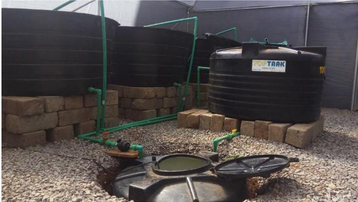
Figure 3.2: The RAS showing the production tanks, biofilter tank and sup tank among other components
