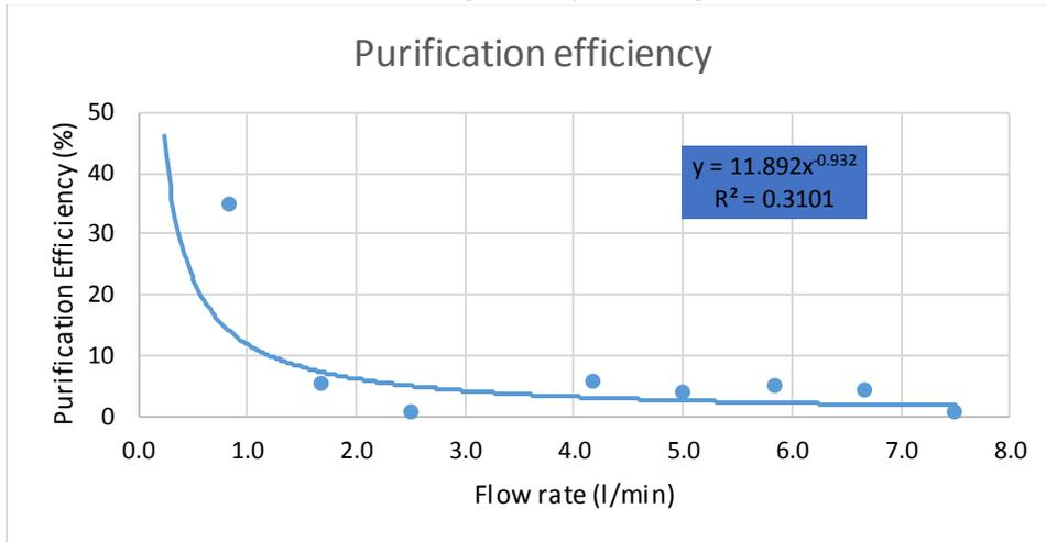
Figure 3.14: Variation of purification efficiency with flow rate at 4kg/m<sup>3</sup> stocking density
