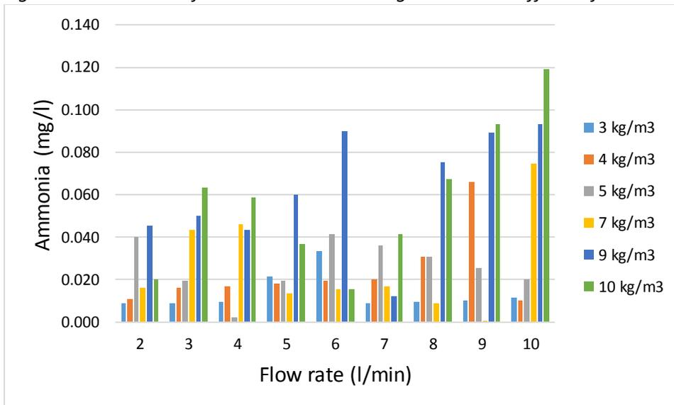
Figure 3.5: Variation of Ammonia with flow rate at different stocking densities
