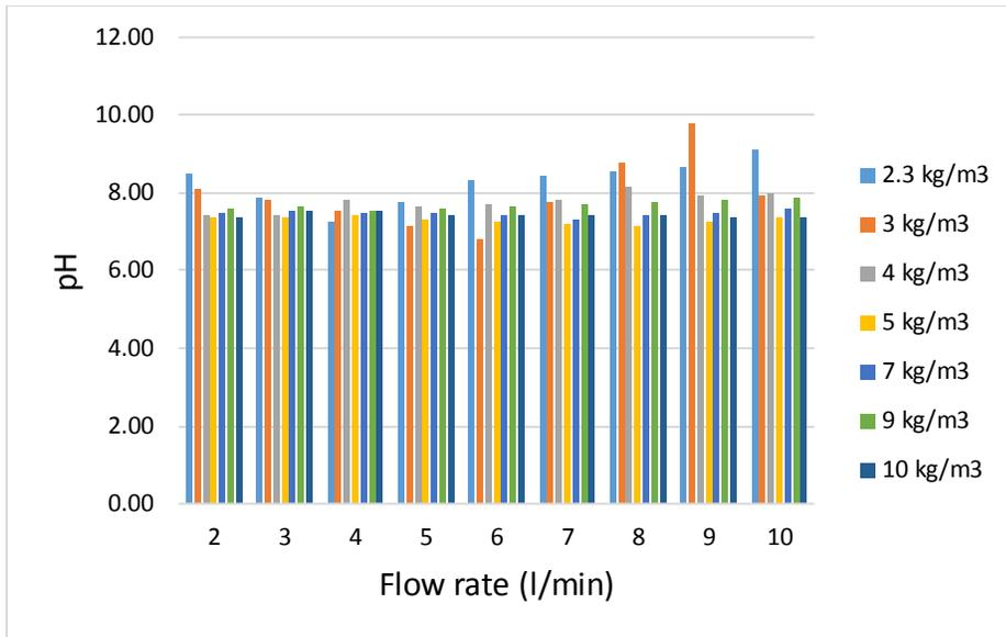
Figure 3.12: Variation of pH with stocking density in the production tank.
