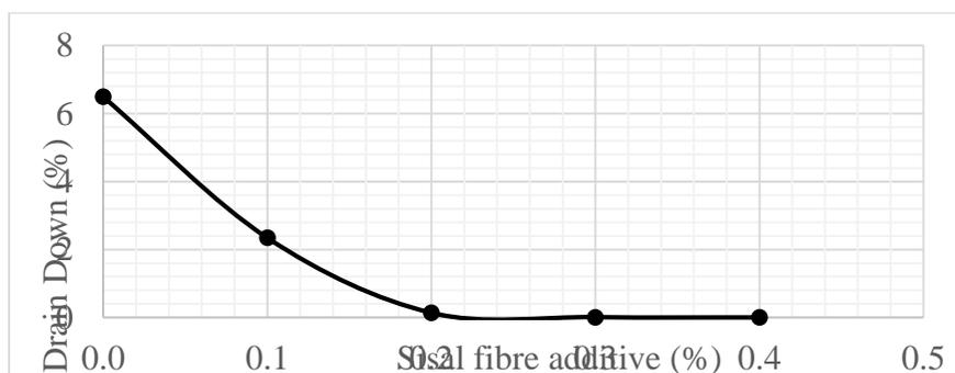
Figure 3(a): Variation of draindown with different percentages of sisal fibre.
